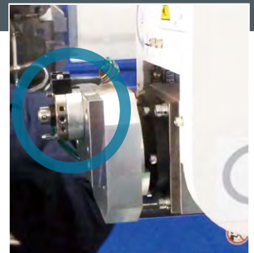
Application example of using a robotic hand changer for chuck plate change
